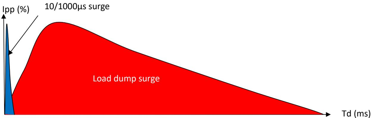
Figure 1. Load dump vs. 10/1000 $\mu$ s surge energy
