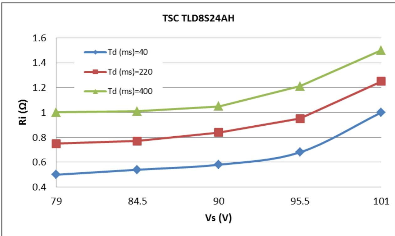
Figure 4. TLD8S24AH SOA (ISO 16750-2 Load dump Test A) Test A
