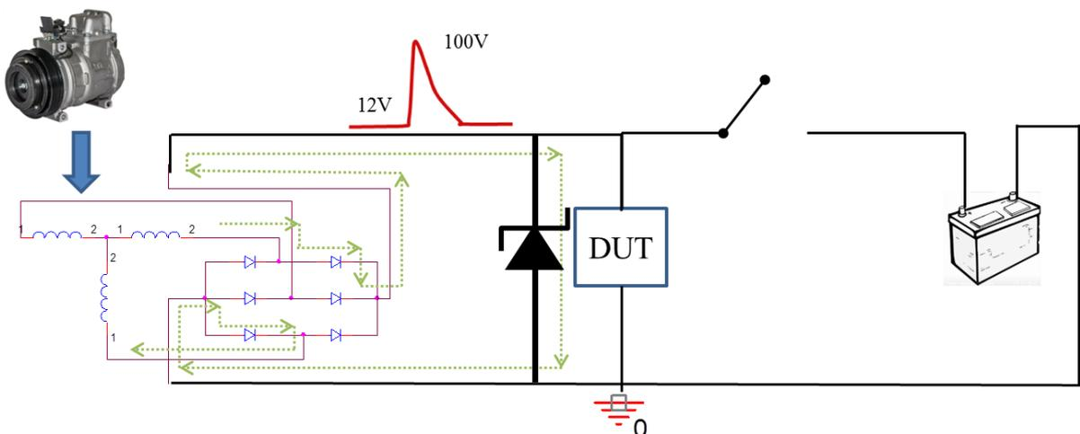
Figure 2. ISO 16750-2 Load dump Test A
