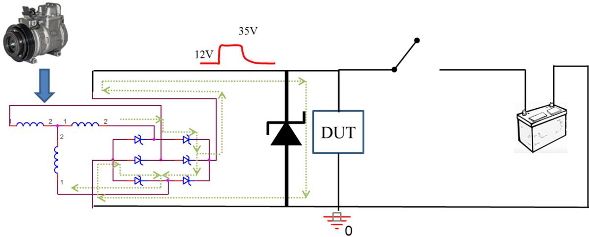
Figure 3. ISO 16750-2 Load dump Test B
