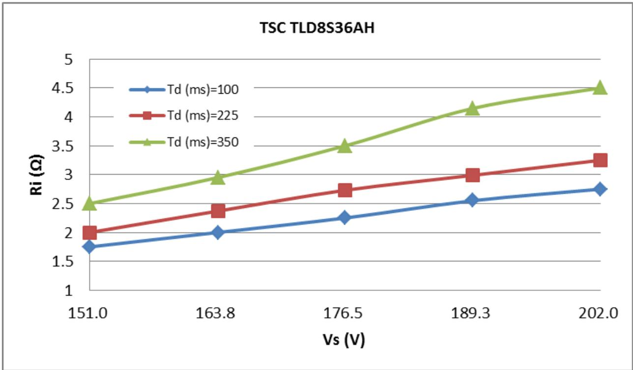
Figure 5. TLD8S36AH SOA (ISO 16750-2 Load dump Test A) Test A
