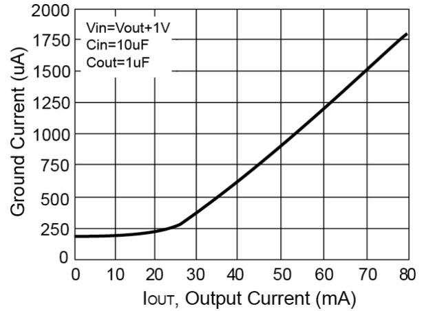
**Figure 2. Ground Current vs. Output Current**
