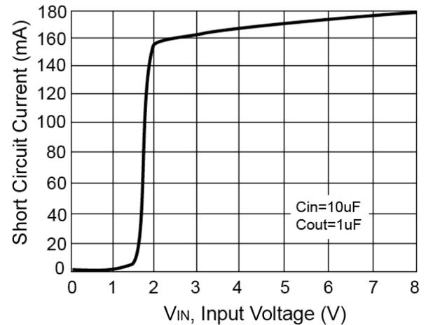
**Figure 4. Short Circuit Current vs. Input Voltage**
