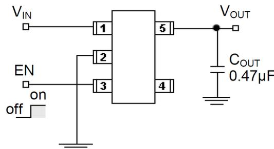
EN may be connected to  $V_{IN}$  pin to regulation ON
