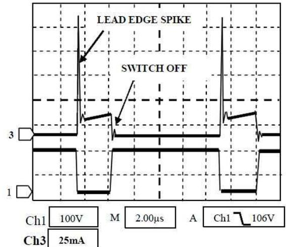
**Figure 2. Switch-On Transition**
