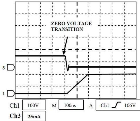
**Figure 1. Switch-Off Transition**
