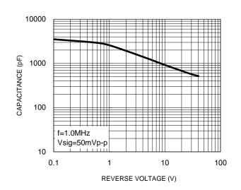
Fig.3 Typical Reverse Characteristics
