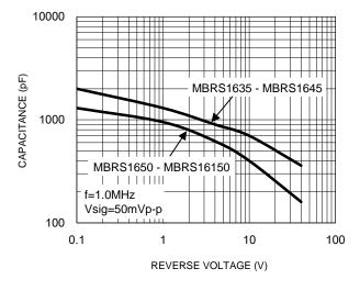
Fig.2 Typical Junction Capacitance
