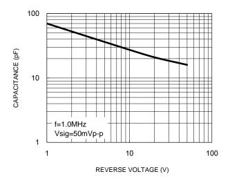
Fig.2 Typical Junction Capacitance
