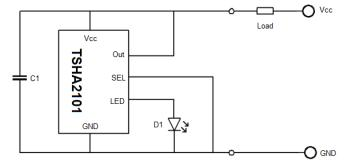
2-wire application circuit with Pull-up load
